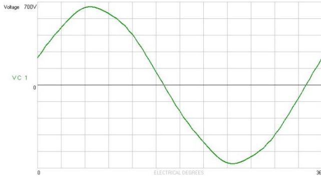
Fig. 12a Output Voltage Waveform for Sinewave Filter tuned to 180 Hz operating at 2 kHz Switching Frequency
