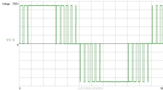
Fig. 11a Inverter Output PWM Voltage Waveform at 2 kHz Switching Frequency
