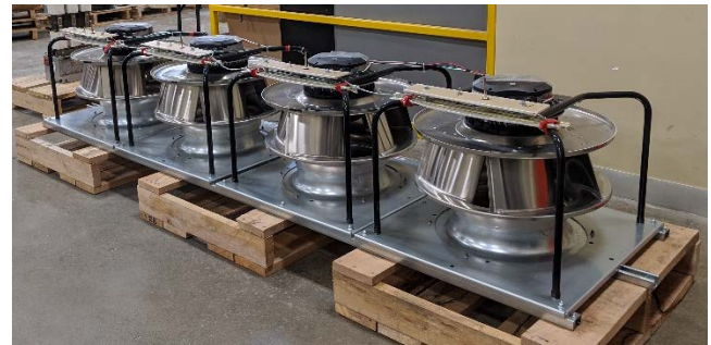
Fig. 9: Array of 4 x 3.75 HP EC fans during factory testing
