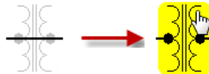
Figure 4-3: Hovering over the Generator/Utility Transformer icon to enter the utility transformer data.
